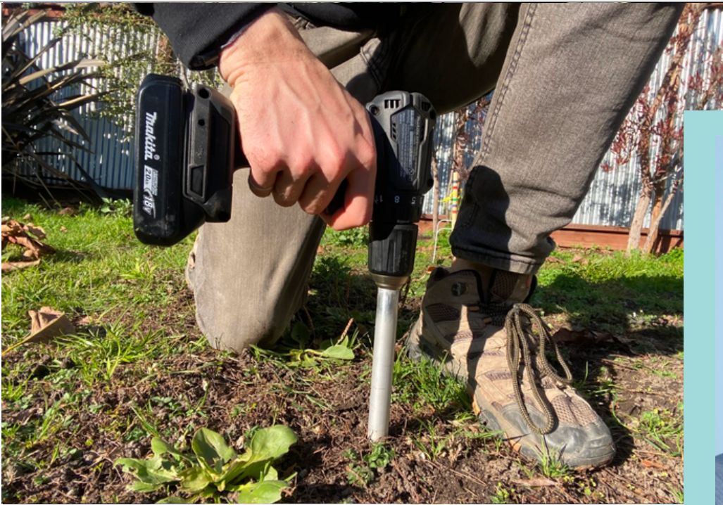
Yard Stick created a hand-held soil probe to measure carbon soil levels onsite. Yard Stick PBC
